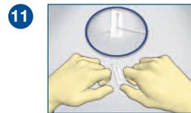
11 After the delivery tubing has primed, make certain the Slide Clamp is in the 'closed' position.
