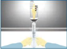
Place the end of syringe plunger on work surface. Keeping the unit vertical, grasp syringe barrel or flanges and push slowly downward on the syringe to gradually force fluid into the Elastomeric Reservoir. Do not grasp the Multirate Infusor device Housing during filling. To fill the Multirate Infusor to the desired volume, steps 2-4 may need to be repeated.
