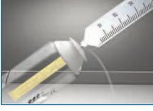
Insert the tip of the filled syringe or filling device into the Fill Port and turn to lock.\*
