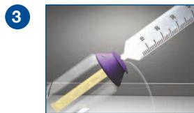
3 Remove Fill Port Cap, retaining it for later use. Beginning with the diluent filled syringe, **gently** insert the tip of the syringe into the Fill Port and turn clockwise to lock.\* (Do not attach a needle to the syringe as this will damage the Fill Port.)
