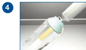
4 **Gently** insert the syringe tip into the Fill Port and turn it clockwise to lock.\*
