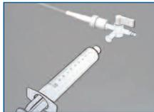
Attach a luer adaptor or stopcock to the Multirate Infusor Luer Lock Connector.
