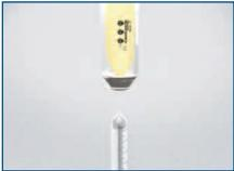
After the Multirate System is filled, remove syringe.
