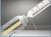
Insert tip of filled syringe into Fill Port and turn gently to lock.\*
