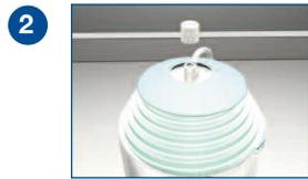
2 With the delivery tubing in place, remove the Fill Port Cap and retain for later use.
